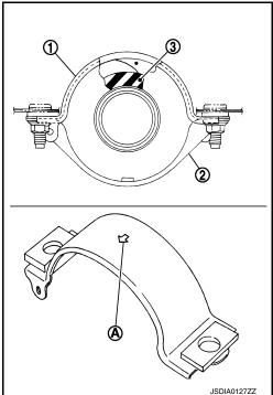
• Align matching marks (A) to install propeller shaft flange yoke and transfer companion flange.
