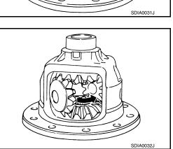
18. Remove pinion mate shaft.
