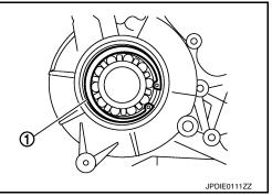
Install main shaft assembly to rear case with the drift (A) [SST: ST35321000 ( — )].
