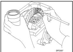
Rotate drive gear back and forth several times, check drive pinion gear to drive gear tooth contact.
