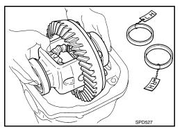
4. Insert left and right original side bearing adjusting washers in place between side bearings and gear carrier.
