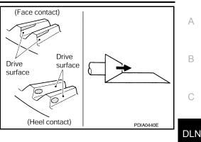
If the tooth contact is near the flank (flank contact), or near the toe (toe contact), thin pinion height adjusting washers to move drive pinion farther from drive gear.
