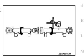
Propeller shaft runout measuring point (Point "△")
