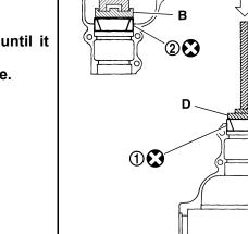
2. Temporarily install pinion height adjusting washer (1).
