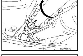
Propeller shaft runout measuring point (Point "△")
