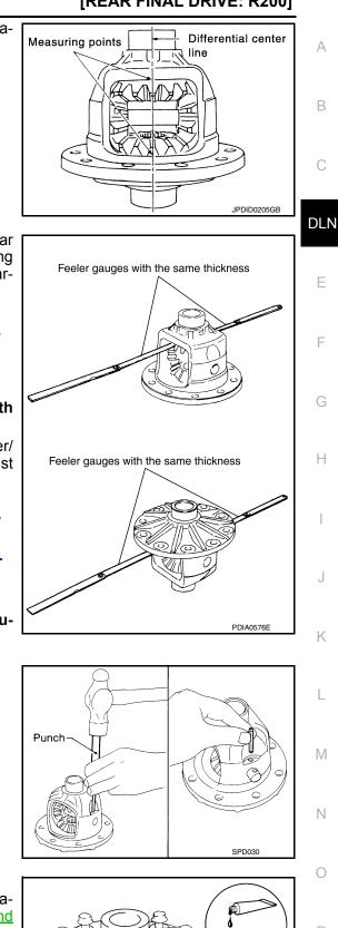
b. Using feeler gauge, measure the clearance between side gear back and differential case at 3 different points, while rotating side gear. Average the 3 readings, and then measure the clearance of the other side as well.
