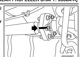
6. Loosen mounting nuts (1) of center bearing mounting brackets (upper/lower).
