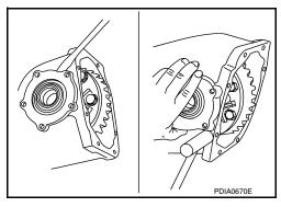
7. Remove differential case assembly from gear carrier.
