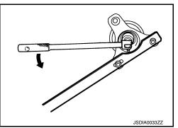
Put matching mark (B) on the end of drive pinion. The matching mark should be in line with the matching mark (A) on companion flange (1).
