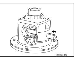
6. Measure side gear end play. If necessary, select the appropriate side gear thrust washers.
