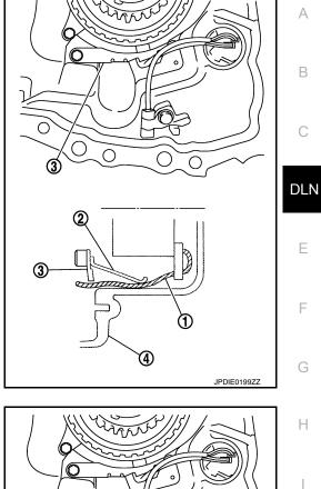
11. Install transfer fluid temperature sensor (1) to rear case.
