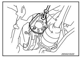
5. Remove side oil seal, using a suitable tool. CAUTION: Never damage gear carrier.
