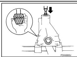
9. Remove pinion rear bearing inner race and pinion height adjusting washer with replacer (A) (commercial service tool).
