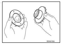
3. Install side gears and thrust washers into differential case. CAUTION:
