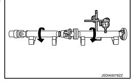
Propeller shaft runout measuring point (Point "△")
