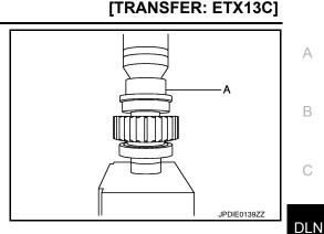
Set drive chain to front drive shaft. **CAUTION:** Identification mark (A) of drive chain should be in the side of front bearing (1) of front drive shaft.
