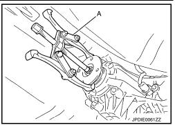
5. Remove the rear oil seal with the puller (A) [SST: KV381054S0 (J-34286)]. CAUTION:
