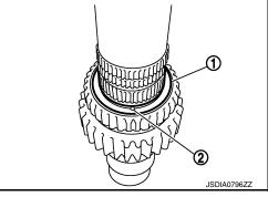
5. Install circlip (1) to notch (A) of the electric controlled coupling.
