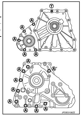
Remove front case (1) from rear case by levering it up with a suitable tool.
