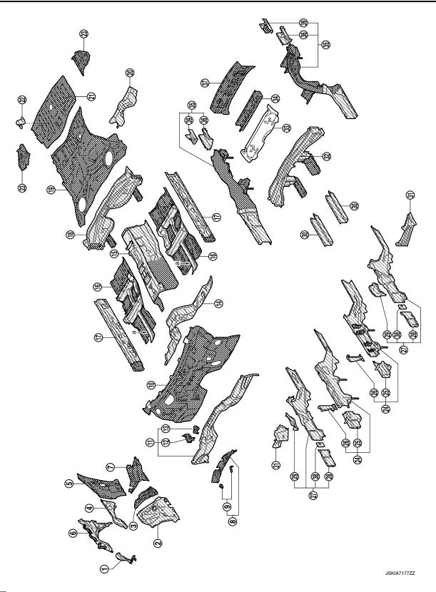
Both sided anti-corrosive precoated steel sections
