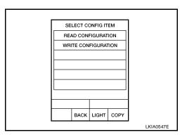
Configuration of current BCM is printed out automatically. A listing of manual setting items and auto setting items will be displayed. Auto setting items are preset and cannot be changed. Manual setting items can be set by using WRITE CONFIGURATION PROCEDURE. Refer to <a href="BCS-16">BCS-16</a>, "WRITE CONFIGURATION PROCEDURE".
