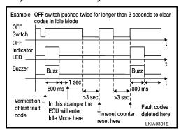
Example: Display fault code: 2 3: OFF switch failure
