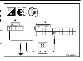
3. Check continuity between combination meter harness connector M24 terminal 27 (O/B) and ground.
