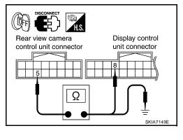
Rear view camera control unit connector
