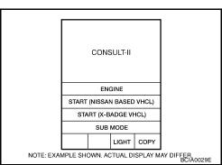
3. Touch "REARVIEW CAMERA" on "SELECT SYSTEM" screen. If "REARVIEW CAMERA" is not indicated, go to GI-39, "CONSULT-II Data Link Connector (DLC) Circuit".
