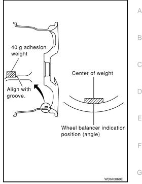
c. If calculated balance weight value exceeds 50 g (1.76 oz), install two balance weight sheets in line with each other as shown.
