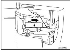
5. Install the in-cabin microfilter cover.
