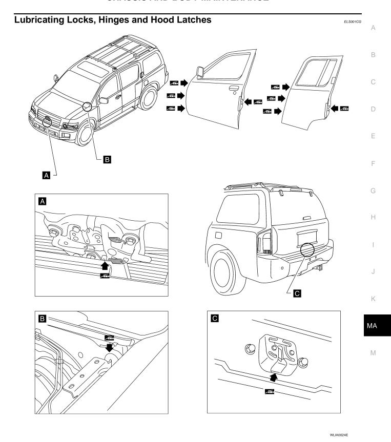
Lubricate the locks, hinges, and latches at the locations as shown. Refer to MA-11, "Fluids and Lubricants" .
