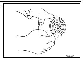
3. Screw the oil filter manually until it touches the installation surface, then tighten it by 2/3 turn. Or tighten to specification.
