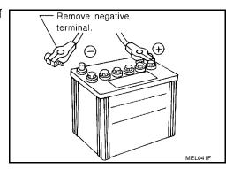
Check the charge condition of the battery.
