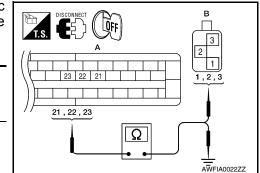
2. Measure the continuity between the ABS actuator and electric unit (control unit) harness connector E125 (A) and body ground.
