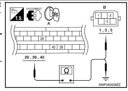
Measure the continuity between ABS actuator and electric unit (control unit) harness connector E125 (A) and body ground.
