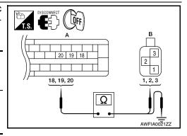
Measure the continuity between the ABS actuator and electric unit (control unit) harness connector E125
