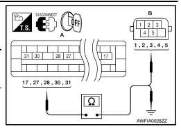
Measure the continuity between ABS actuator and electric unit (control unit) harness connector E125 (A) and body ground.
