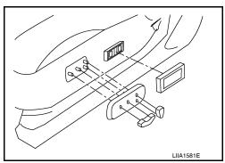
2. Remove the power seat and power lumbar switches.
