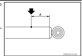
3. Position the drilled hole downward and drain oil by moving the piston rod several times. CAUTION:
