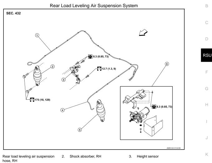
4. Rear load leveling air suspension 5. Shock absorber, LH hose, LH
