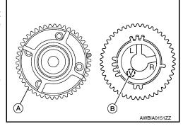
3. Install the crankshaft sprockets for both banks.
