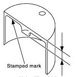
Valve lifter thickness  $_{\rm SEM758G}$
