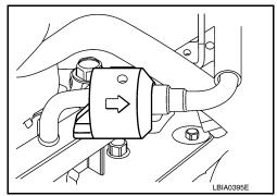
Remove quick connector cap (engine side only).
