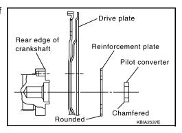
Inspection After Disassembly
