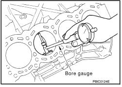
If measured value exceeds the repair limit, or if there are scratches and/or seizure on the cylinder inner wall, hone or bore the inner wall.
