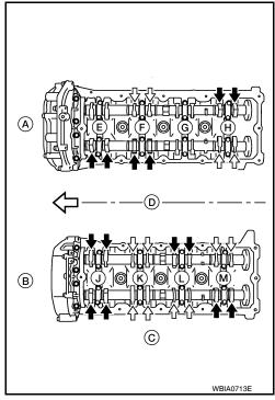
Measure valve clearance using suitable tool. Refer to <u>EM-108</u>, <u>"Standard and Limit"</u>.
