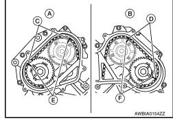
11. Remove the chain tensioner (LH) using the following steps.
