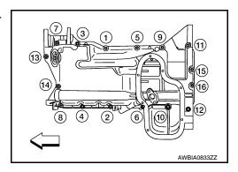
b. Remove the oil pan (upper) from the cylinder block by prying it at the points shown, using suitable tool.
