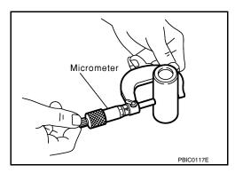
Piston and Piston Pin Clearance
