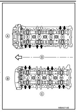
Measure valve clearance using suitable tool. Refer to <u>EM-108</u>, <u>"Standard and Limit"</u>.
