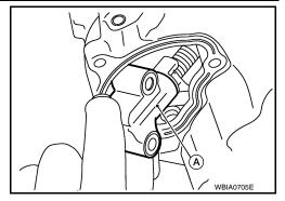
14. Loosen camshaft sprocket bolts as shown and remove camshaft sprockets.
