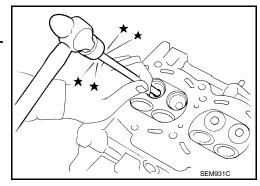
3. Ream the cylinder head valve guide hole using suitable tool.
