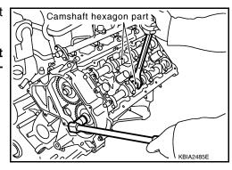
15. Remove the RH (A) front cover bolts and LH (B) front cover bolts.
