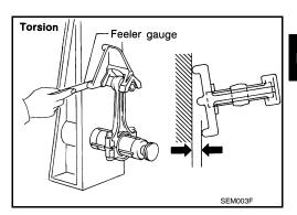
If measurement exceeds the limit, replace connecting rod assembly.
