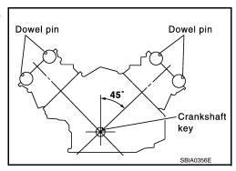
2. Install the camshaft sprockets.
