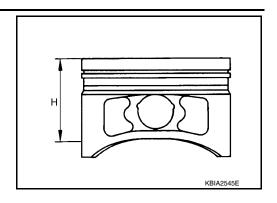
Piston to Cylinder Bore Clearance
