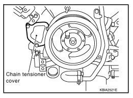
13. Remove the chain tensioner (RH) using the following steps.
