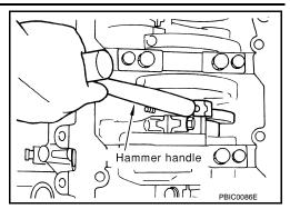
Remove connecting rod bearings.
