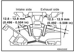
6. Ream the cylinder head valve guide using suitable tool.
