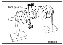
Taper: Difference between A and B Out-of-round: Difference between X and Y PBIC1685E
