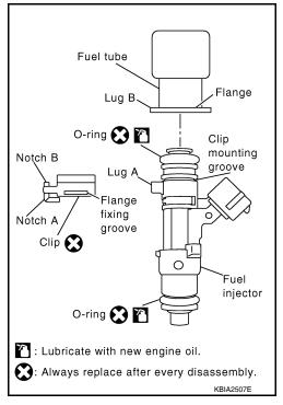
4. Install fuel tube and fuel injector assembly to intake manifold.
