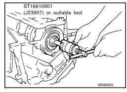
4. Cut away liquid gasket and remove rear oil seal retainer using Tool. Refer to <a href="EM-4">EM-4</a>, "Precaution for Liquid Gasket".
