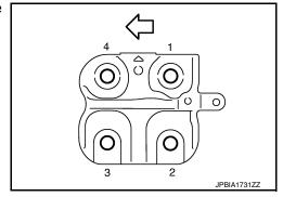
13. Remove the engine mount bracket (front).
