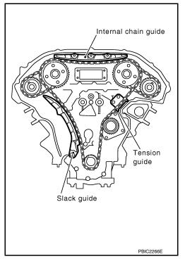
Remove timing chain (primary) and crankshaft sprocket. CAUTION:
