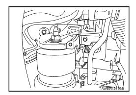
12. Loosen the engine mount bracket (front) bolts in the reverse order shown.
