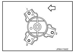
15. Remove the engine mount insulator (front).
