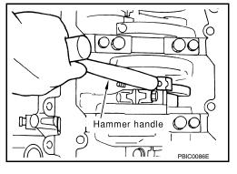
13. Remove the connecting rod bearings.
