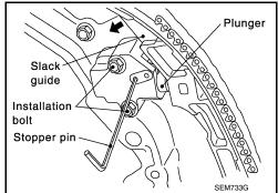
8. Remove internal chain guide, tension guide and slack guide. **NOTE:**
