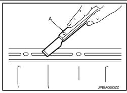
Attach the liquid gasket tube to the suitable tool.
