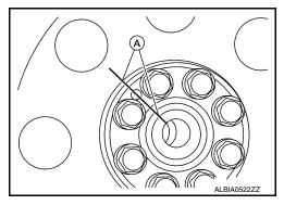
• Install the drive plate and the reinforcement plate in the direction as shown.
