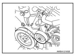
b. Check that the valve lifters on No.1 cylinder are loose and valve lifters on No.4 are tight. If not, turn the crankshaft one full revolution (360°) and align as shown.
