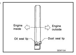
a. Install the new front oil seal so that it becomes flush with the face of front timing chain case using suitable tool.
