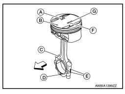
Piston and Piston Pin Interference Fit Standard Interference Fit = (Dp) – (dp)
