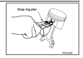
b. Heat the pistons to  $60^{\circ}$  -  $70^{\circ}$ C ( $140^{\circ}$  -  $158^{\circ}$ F).
