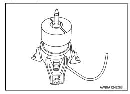
2. Install the engine mount insulator (front) bolts and tighten to specification in the order shown.
