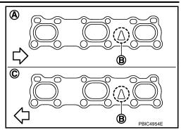
3. Install the exhaust manifold (RH) nuts and tighten to specification in the order shown.
