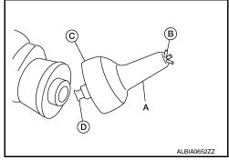
d. Apply sealant to rear oil seal retainer as shown.
