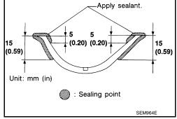
3. Install the front cover gasket and rear oil seal retainer gasket as shown.
