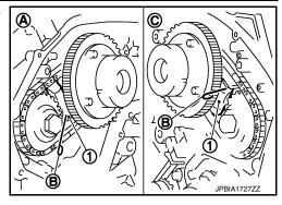
6. Install the crankshaft sprocket on the crankshaft.
