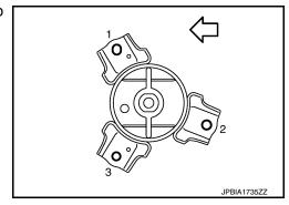
3. Install the engine mount bracket (front) to the engine block.
