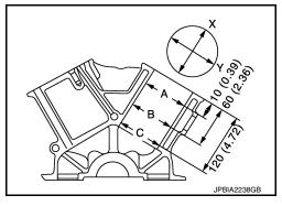
5. Cylinder bore size is determined by adding piston-to-bore clearance to piston diameter (A).
