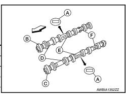
• Position the camshaft dowel pins (A) as shown.
