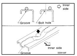
2. Install the lower oil pan. Tighten the lower oil pan bolts in order as shown.
