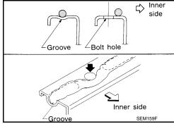
Install new O-rings on the cylinder block and oil pump body. CAUTION:
