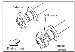
Follow your identification marks made during removal or follow the identification marks that are present on the new camshafts components for proper placement and direction of the components.
