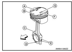
c. Install the snap ring into the front of the piston pin-groove.
