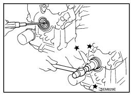
24. Remove all old liquid gasket from all the bolt holes and bolts.
