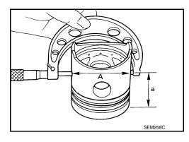
4. Check that piston-to-bore clearance is within specification.
