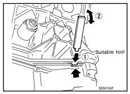
13. Remove the O-ring seals from the bottom of the cylinder block and oil pump housing. Use new O-rings for installation. CAUTION:
