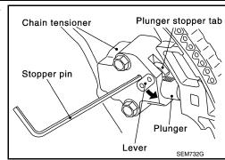
Insert stopper pin into timing chain tensioner (primary) body hole to hold lever, and keep the tab released. An Allen wrench [1.2 mm (0.047 in)] is used for a stopper pin as an example.
