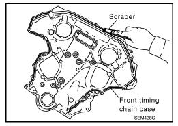
8. Remove all old Silicone RTV Sealant from all the bolt holes and bolts.
