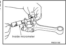
CONNECTING ROD BUSHING OIL CLEARANCE (SMALL END)
