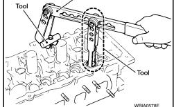
5. Remove valve oil seal using Tool.
