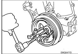
Remove front oil seal from front cover using a suitable tool.
