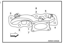
14. Remove the exhaust manifold (RH).
