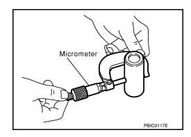
Connecting Rod Bushing Oil Clearance (Small End)
