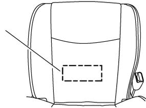
**F** • Climate controlled seat control unit (passenger seat)
