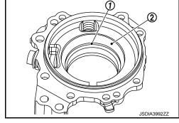
Install the transfer cover to the transfer case, and apply anti-corrosive oil onto thread and seats on the mounting bolts. Then tighten mounting bolts to the specified torque.
