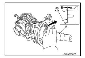
4. Apply liquid gasket (1) to mating surface of coupling cover.
