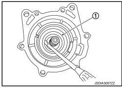
8. Remove side oil seal (1), using a oil seal remover. CAUTION:
