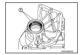
Remove baffle plate (1).
