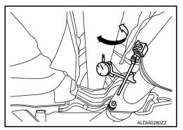
• Propeller shaft runout measuring point (Point "△").
