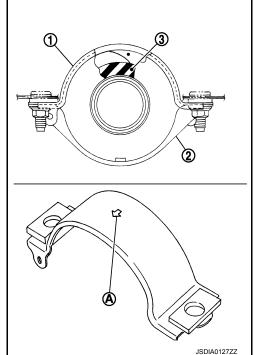
• After tightening the bolts and nuts to the specified torque, check that the bolts (3) on the flange side are tightened as shown.
