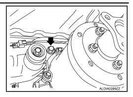
11. Remove rear final drive nut (←) at rear suspension member, and remove final drive from vehicle.
