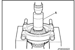
6. Remove ring gear bearing inner race (transfer case side) from ring gear shaft with the drift (A) [SST: ST33061000 (J-8107-2)] and puller (commercial service tool).
