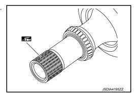
b. Wrap piece of vinyl to spline part only indicated in the figure. [(A): limit line]
