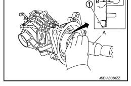
8. Apply liquid gasket (1) to mating surface of coupling cover.
