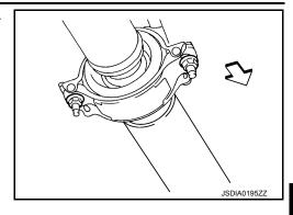
5. Remove propeller shaft assembly nuts and bolts.Refer to <a href="DLN-92">DLN-92</a>, "Exploded View".
