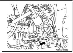
2. Install side oil seal (carrier side) until it becomes flush with the carrier end, using Tool (A) and Tool (B).
