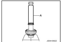
Apply multi-purpose grease to spline part indicated in the figure.
