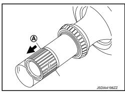
Measure the total preload without oil seals of transfer cover and transfer case.
