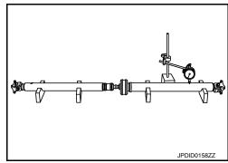
Propeller shaft runout measuring point (Point "△").
