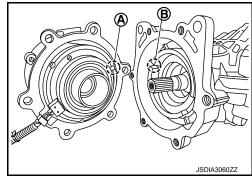
Press the electric controlled coupling pin to check that it is positioned in the groove of the final drive assembly as shown in the figure.
