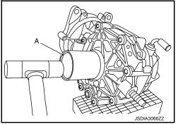
3. Install side oil seal (carrier side) until it becomes flush with the carrier end, using the drift (A) and drift bar (B).
