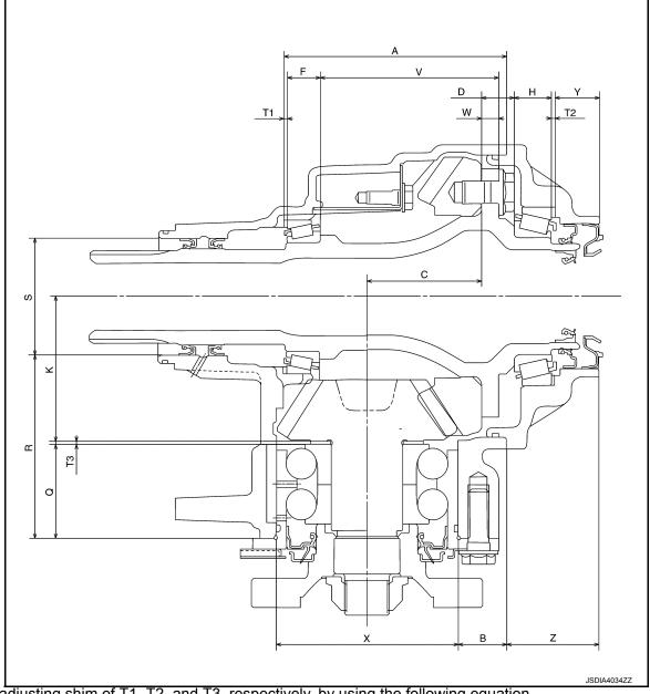
Select adjusting shim of T1, T2, and T3, respectively, by using the following equation.
