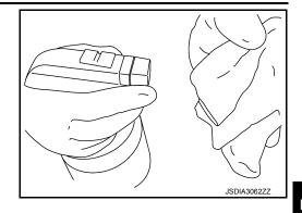
2. Wipe the mounting surface of electric controlled coupling five times.
