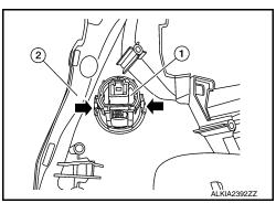
3. Release the pawl on each side and remove the NATS antenna amp from the push-button ignition switch.
