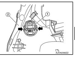
3. Release the pawl on each side and remove the push-button ignition switch from the NATS antenna amp.
