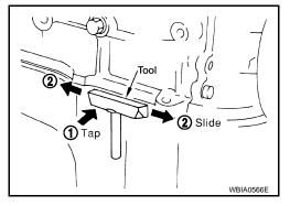
38. Remove the water pump cover and chain tensioner cover from the front timing chain case using Tool.
