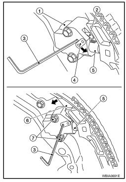
Remove primary timing chain and crankshaft sprocket. CAUTION:
