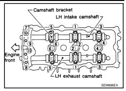
12. Measure difference in levels between front end faces of camshaft No. 1 bracket and cylinder head.
