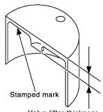
Valve lifter thickness SEM758G
