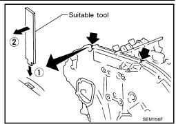
Use the Tool by tapping (1) and sliding (2) using a plastic hammer to remove the lower oil pan from the upper oil pan.
