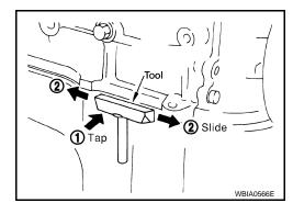
7. Remove the IVT control cover bolts in the order as shown and remove the IVT control covers.
