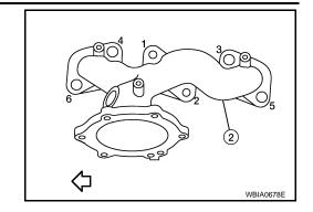
• Install the bank 1 (1) and bank 2 (2) three way catalyst support bolts in the order as shown.
