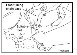
7. Loosely install the front timing chain case bolts.
