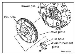
Install the driveplate and reinforcement plate in the direction shown.
