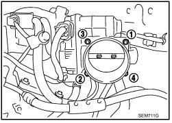
14. If necessary, remove the intake manifold collector (upper) bolts in the order as shown, using power tool and remove the intake manifold collector (upper).
