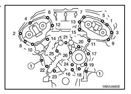
b. Cut the sealant using Tool (A) and remove the rear timing chain case.
