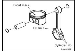
Install the piston to the connecting rod.
