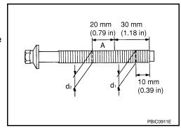
OUTER DIAMETER OF CONNECTING ROD BOLTS
