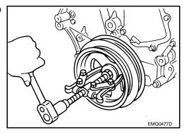
Remove front oil seal from front timing chain case. CAUTION:
