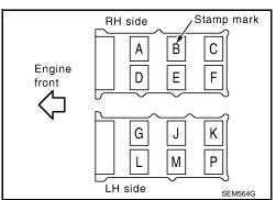
11. Tighten the camshaft brackets in four steps in the order as shown.
