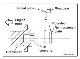
21. Secure the driveplate using Tool.
