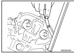
13. Install the IVT control solenoid valves with new gaskets.
