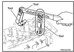
4. Remove valve oil seal using Tool.
