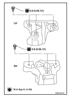
• Install the three way catalyst manifolds heat shield bolts.
