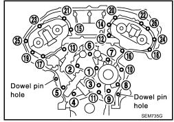
After all bolts are initially tightened, retighten them to the specification in the order as shown.
