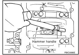
Remove the connecting rod bearings.
