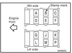
8. Tighten the camshaft brackets in the four steps, as shown.
