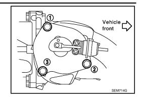
• If removed, tighten the intake manifold collector (upper) bolts in the order as shown.
