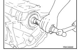
· Install pilot converter as shown.
