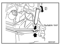
22. Remove the O-ring seals from the bottom of the cylinder block and oil pump housing, use new O-rings for installation.
