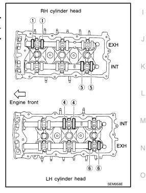
12. If all valve clearances are within specification, installation of the remaining components is in the reverse order of removal. If the valve clearances are out of specification, adjust the valve clearances. Follow the "VALVE ADJUSTING" procedure.
