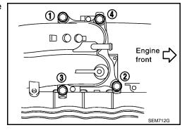
• If removed, install the electric throttle control actuator bolts in the order as shown. Install gasket with three protrusions facing down.
