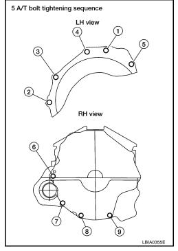
Install converter to drive plate bolts.
