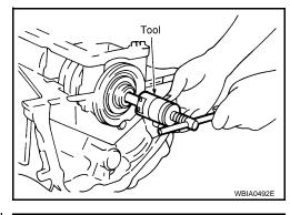
11. Cut away liquid gasket using Tool and remove rear oil seal retainer. Refer to <a href="EM-4">EM-4</a>, "Precaution for Liquid Gasket".
