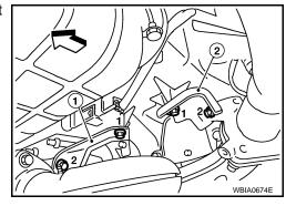
Install the exhaust manifold heat shield bolts.
