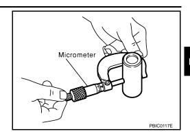
Connecting Rod Bushing Oil Clearance (Small End)
