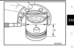
Check that piston-to-bore clearance is within specification.
