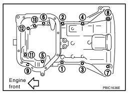
Install the four upper oil pan to transaxle bolts. Refer to EM-110. "Removal and Installation".
