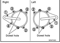
11. Apply liquid gasket and install the water pump cover and the chain tensioner cover.
