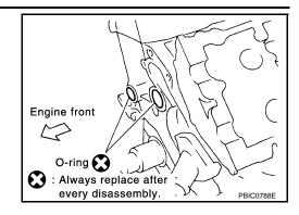
28. If necessary, remove the water pump. Refer to <u>CO-19.</u> "Removal and Installation".
