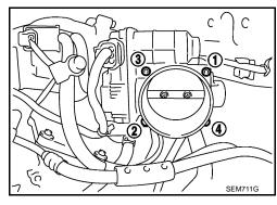
Install the intake manifold collector (lower) bolts in the order as shown.
