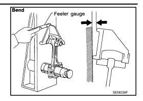
• If it exceeds the limit, replace connecting rod assembly.
