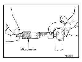
Piston and Piston Pin Interference Fit
