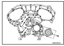
Apply Silicone RTV Sealant to rear timing chain case as shown.
