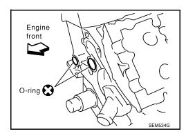
15. Install RH (1) and LH (2) new O-rings (3) on the cylinder heads.
