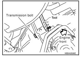
c. Loosen crankshaft pulley bolt and locate bolt seating surface at 10 mm (0.39 in) from its original position.
