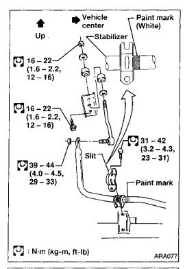
Install stabilizer bar with ball joint socket properly placed.
