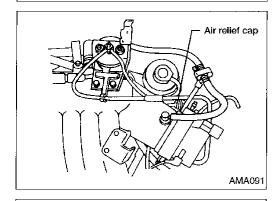
18. Install 1 meter (40") of 6 mm (0.24 in) I.D. heat resistant hose (clear if available, minimum temperature rating 105°C/220°F) to heater pipe air relief.
