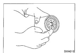
2. Clean oil filter mounting surface on cylinder block. Coat rubber seal of new oil filter with engine oil.
