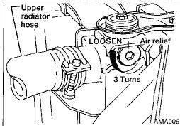
17. Remove heater pipe air relief cap.
