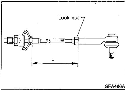
7. Adjust toe-in by varying the length of steering tie-rods.
