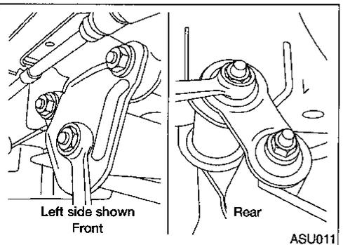
8. Tighten spring shackle nuts, front eye bolt nuts and upper pin nuts and shock absorber nuts. Refer to SU-18.
