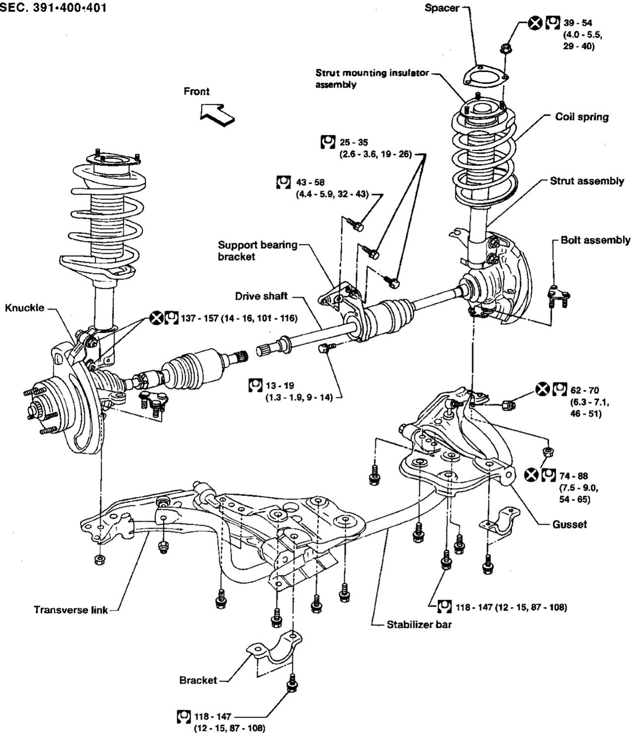
When installing rubber parts, final tightening must be carried out under unladen condition\* with tires on ground.
