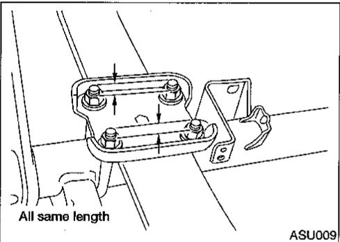
3. Install leaf spring assembly aligning spring center bolt with the hole in lower seat.
