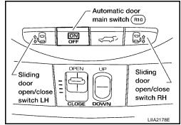
7. Press and HOLD the overhead Sliding Door Open/Close Switch of the door being initialized until the door completely closes and stops, then release the switch.
