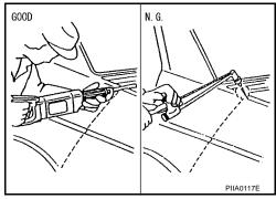
• When welding HSS panels, use spot welding whenever possible in order to minimize weakening surrounding areas due to heat.
