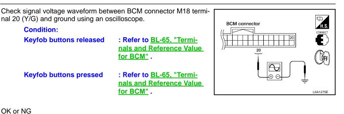
>> Remote keyless entry receiver signal power supply, ground and signal circuits are OK. Replace OK BCM. Refer to BCS-19, "Removal and Installation of BCM".
