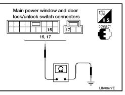
4. Check continuity between power window and door lock/unlock switch RH connector D105 terminal 11 and ground.
