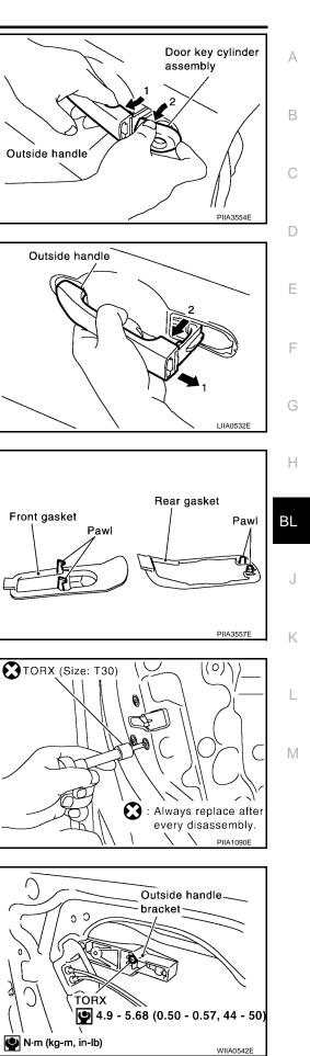
9. While pulling outside handle bracket, slide toward rear of vehicle to remove outside handle bracket and door lock assembly.
