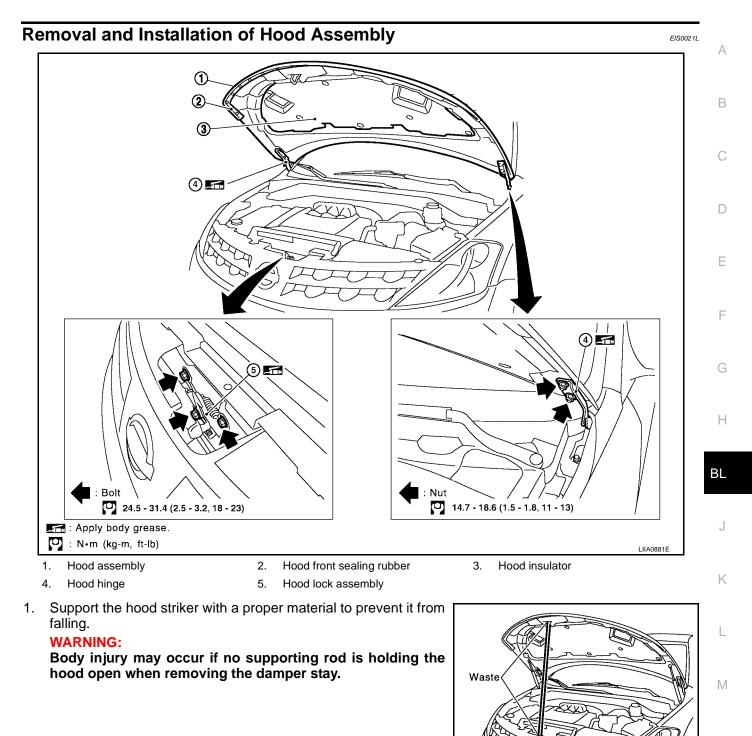
2. Remove the hinge nuts on the hood to remove the hood assembly.
