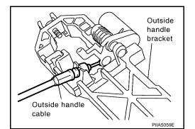
While pulling outside handle, slide toward rear of vehicle to remove outside handle and door lock assembly.
