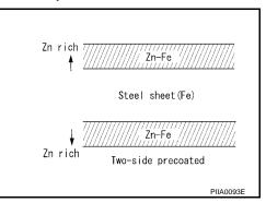
Nissan Genuine Service Parts are fabricated from galvannealed steel. Therefore, it is recommended that GENUINE NISSAN PARTS or equivalent be used for panel replacement to maintain the anti-corrosive performance built into the vehicle at the factory.
