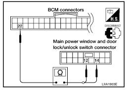
3. Check continuity between BCM connector M18 terminal 22 and power window and door lock/unlock switch RH connector D105 terminal 16.
