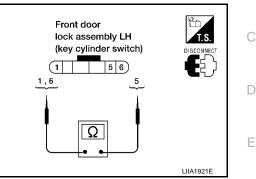
NG >> Replace front door lock assembly LH. Refer to <u>BL-194, "FRONT DOOR LOCK"</u>.
