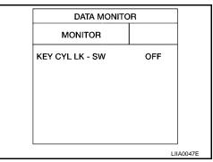
Check front door lock assembly LH (key cylinder switch) ("KEY CYL UN-SW") in "DATA MONITOR" mode for "POWER DOOR LOCK SYSTEM" with CONSULT-II. Refer to <u>GW-40, "DATA</u> <u>MONITOR"</u>.
