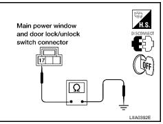
4. Check continuity between power window and door lock/unlock switch RH connector D105 terminal 11 and ground.
