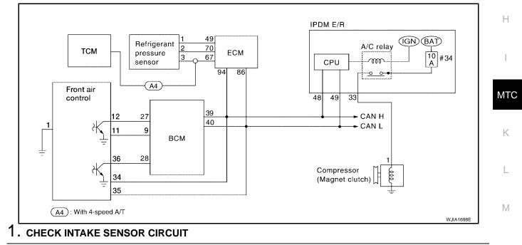
Check intake sensor. Refer to MTC-54, "A/C System Self-diagnosis Function" .
