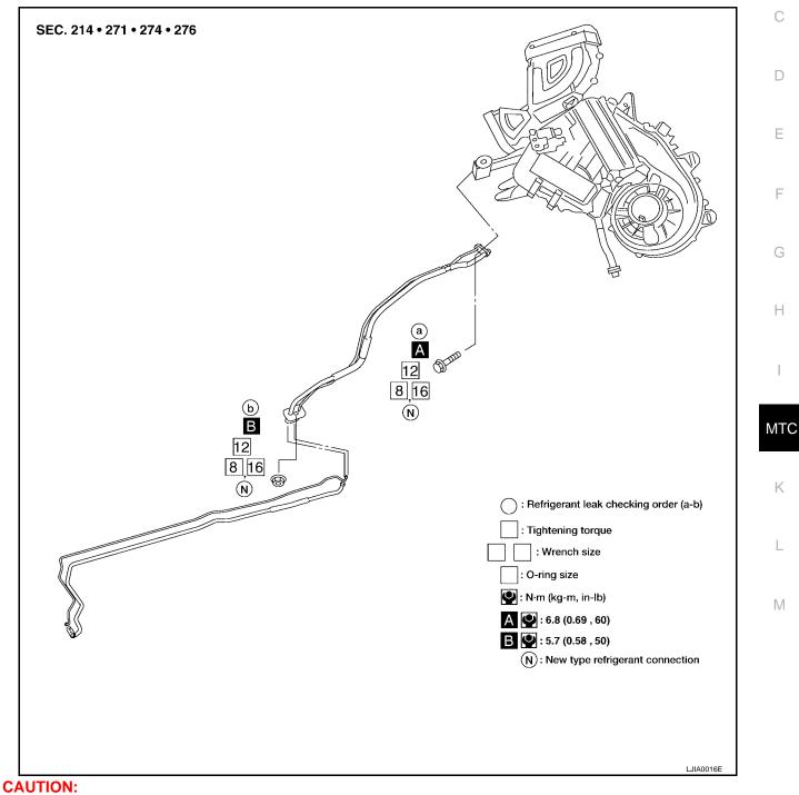
The new and former refrigerant connections use different O-ring configurations. Do not confuse O-rings since they are not interchangeable. If a wrong O-ring is installed, refrigerant will leak at or around the connection.
