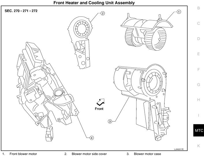
4. Heater core and evaporator case
