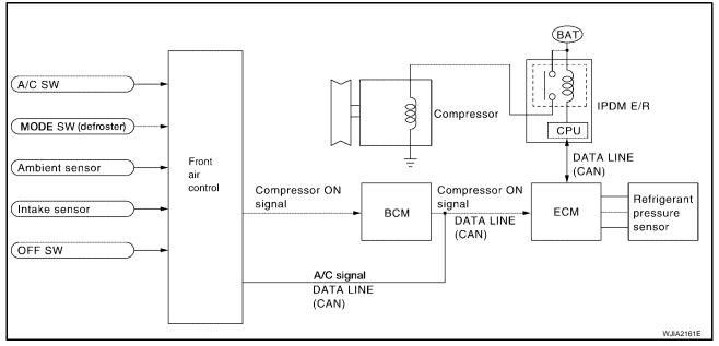
When the A/C switch is pressed, or the mode switch is turned to the defroster position, the front air control outputs a compressor ON signal to BCM.
