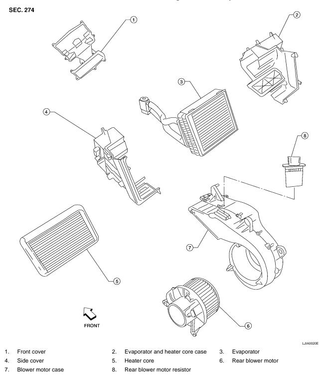
Removal and Installation FRONT HEATER CORE
