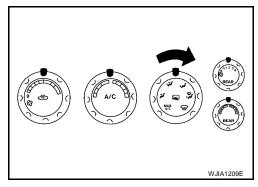
3. Confirm that discharge air comes out according to the air distribution table. Refer to <u>MTC-29, "Discharge Air Flow"</u>.
