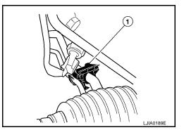
e. Carefully remove the lower section of the high/low pressure pipe (1).
