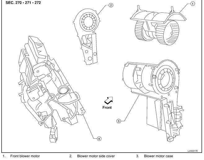
4. Heater core and evaporator case
