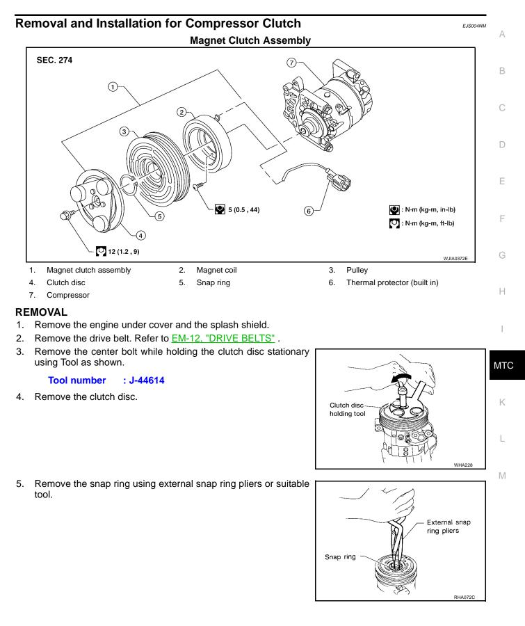
6. Remove the pulley using Tool with a small adapter. Position the small adapter on the end of the drive shaft and the center of the puller on the small adapter.
