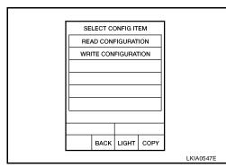
Configuration of current BCM is printed out automatically. A listing of manual setting items and auto setting items will be displayed. Auto setting items are preset and cannot be changed. Manual setting items can be set by using WRITE CONFIGURATION PROCEDURE. Refer to <a href="BCS-21">BCS-21</a>, "WRITE CONFIGURATION PROCEDURE".
