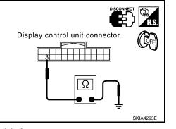
Power Supply and Ground Circuit Inspection for Display Unit
