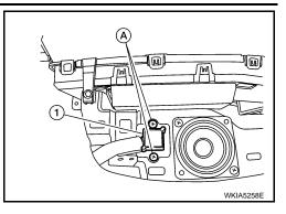
5. Disconnect GPS antenna connector and remove GPS antenna and feeder assembly out the top.
