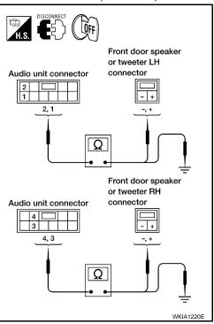
Check continuity between audio unit harness connector M43 terminal and ground.
