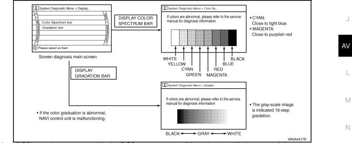
When RGB signal error occurred in the RGB system, tone of the color bar will change as follows.
