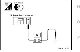
4. Check voltage between BOSE speaker amp. (with BOSE) and ground.
