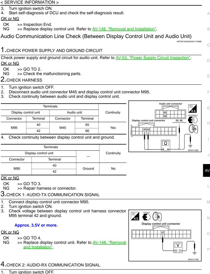
Disconnect display control unit connector M95.
