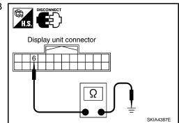
Power Supply and Ground Circuit Inspection for Color Display
