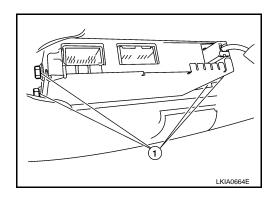
4. Remove satellite radio tuner unit.
