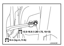
Remove the door-side hinge nuts and bolts, and remove the door assembly.
