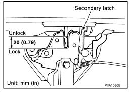
3. Check the hood lock lubrication condition. If necessary, apply "body grease" to the points shown in the figure.
