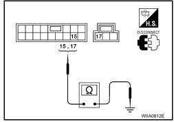
Check continuity between power window and door lock/unlock switch RH connector D105 terminal 11 and ground.
