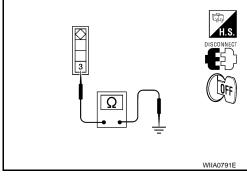
Door Switch Check (With Automatic Back Door System)
