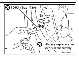
7. Remove the TORX bolt (T30), and remove the outside handle bracket.
