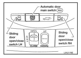
Within 3 seconds after step 3, press the door pillar Sliding Door Open/Close Switch of the door being initialized 10 times within 10 seconds.
