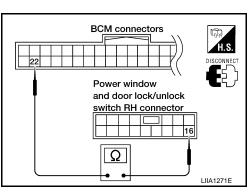
Power Window Serial Link Check Front LH and RH (With Rear Power Vent Windows)
