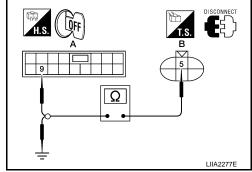
2. Check continuity between front power window motor LH connector and ground.
