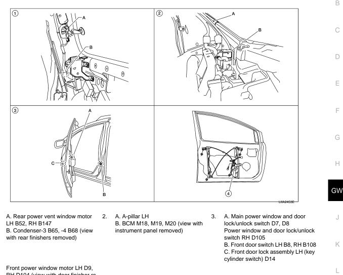
Front power window motor LH D9, RH D104 (view with door finisher removed)
