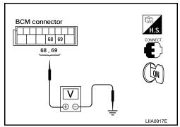
Main power window and door lock/unlock switch connector 17
