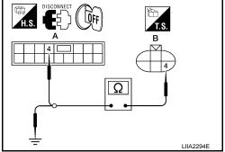
4. Check continuity between front power window motor LH connector and ground.
