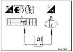
4. Check continuity between front power window motor LH connector and ground.
