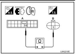
Check continuity between front power window motor LH connector and ground. 4.
