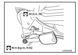
Installation Installation is in the reverse order of removal.
