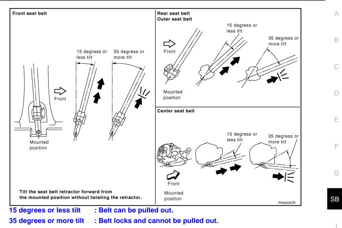
If retractor does not operate within specifications, replace the retractor assembly.
