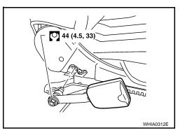
Installation Installation is in the reverse order of removal. Third Row Seat Belt
