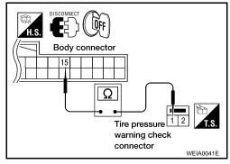
Inspection 4 Hazard Warning Lamp Flashes When Ignition Switch Is Turned On
