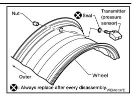
4. Place wheel on turntable of tire machine. Ensure that transmitter is 270 degrees from mounting/dismounting head.
