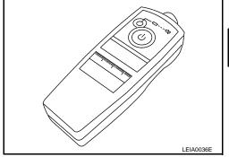
Register the IDs in order from FR LH, FR RH, RR RH and RR LH. When ID registration of each wheel has been completed, a buzzer sounds and the hazard warning lamps flash.
