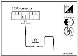
Inspection 3 Warning Lamp Flashes When Ignition Switch Is Turned On
