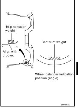
c. If calculated balance weight value exceeds 50 g (1.76 oz), install two balance weight pieces in line with each other (as shown in the figure).
