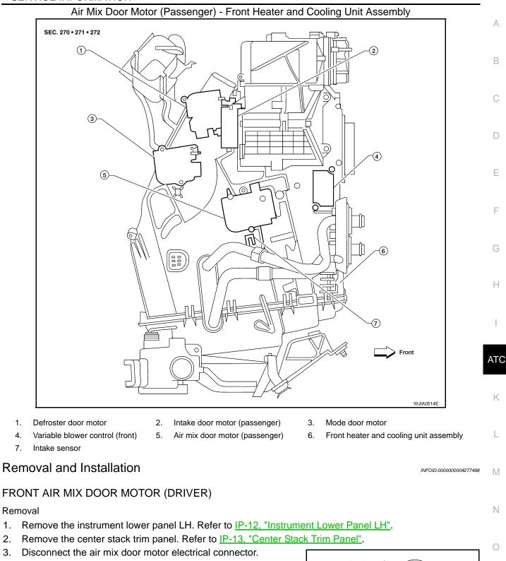
4. Remove the three screws and remove the air mix door motor.
