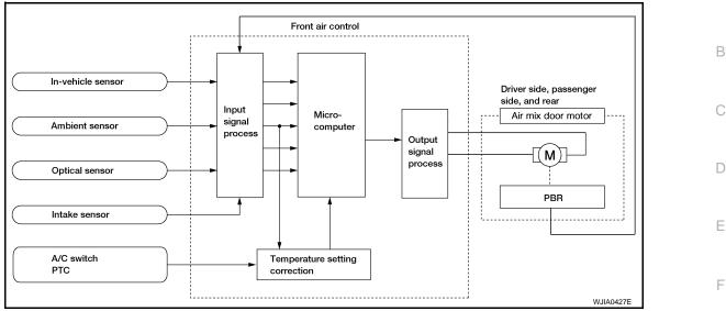
Air Mix Door Control Specification COMPONENT DESCRIPTION
