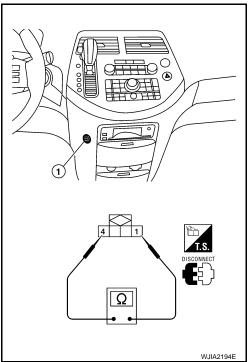
If NG, replace in-vehicle sensor. Refer to <u>ATC-130, "Removal and</u> <u>Installation"</u>.
