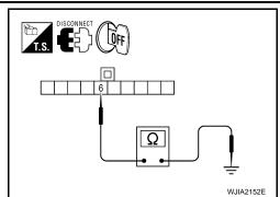
**4.**CHECK REAR AIR CONTROL (REAR) REAR AUX BLOWER POT BETWEEN FRONT AIR CONTROL AND REAR IAR CONTROL REAR
