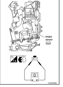
If NG, replace intake sensor. Refer to <u>ATC-132</u>, "Removal and Installation".
