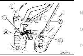
d. Attach the other pipe support clip to the dash panel threaded stud.
