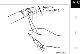
2. When checking for leaks, circle each fitting completely with the probe as shown.
