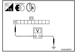
**2.**CHECK REAR AIR CONTROL (FRONT) REFERENCE VOLTAGE
