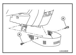
Front heater and cooling unit assembly
