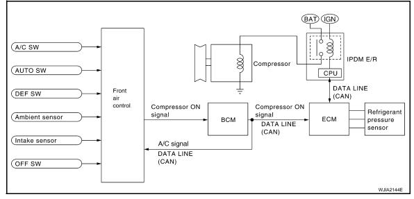
When A/C switch or DEF switch is pressed, front air control outputs compressor ON signal to BCM. BCM sends compressor ON signal to ECM and front air control, via CAN communication line.
