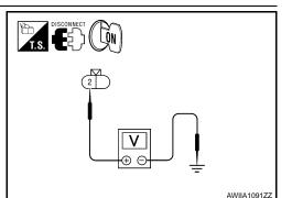
2.CHECK CIRCUIT CONTINUITY BETWEEN AMBIENT SENSOR AND FRONT AIR CONTROL
