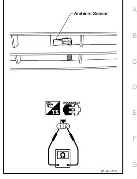
If NG, replace ambient sensor. Refer to <u>ATC-129</u>, "Removal and <u>Installation"</u>.
