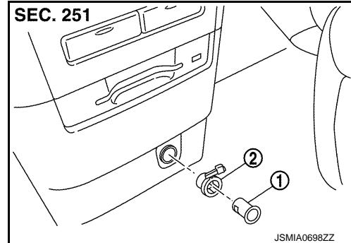
**FRONT POWER SOCKET : Removal and Installation**
