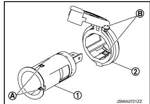
4. Press the ring pawl from the back of the luggage side lower finisher (LH) to remove the ring.
