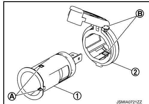
3. Press the ring pawl from the back of the instrument lower cover center to remove the ring.
