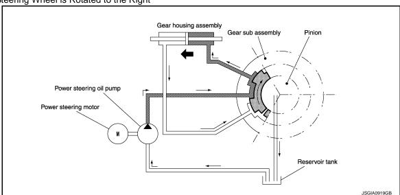
The hydraulic routes open from power steering pump to gear housing right side and from gear housing left side to reservoir tank, providing left direction assist force to the rack.
