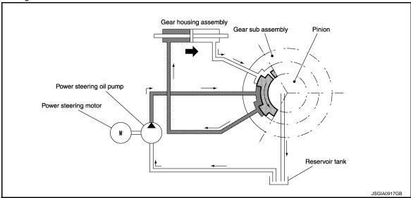
The hydraulic routes open from power steering pump to gear housing left side and from gear housing right side to reservoir tank, providing right direction assist force to the rack.
