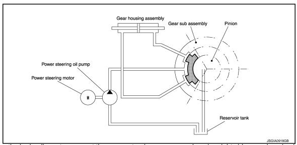
Because the hydraulic routes open at the power steering pump, gear housing right side, gear housing left side, and reservoir tank, the hydraulic pressure applied to the right side and left side of the gear housing is equal and no steering assist force is generated.
