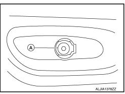
3. Release pawls using a suitable tool (A) and remove rear power window switch finisher (1).
