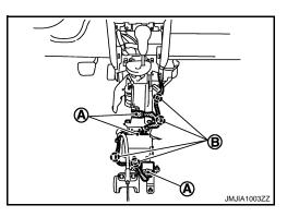
Remove screw (A), and then remove front foot duct RH (1) (with rear foot duct model). Refer to <u>VTL-48</u>, "FRONT FOOT DUCT : Removal and Installation".
