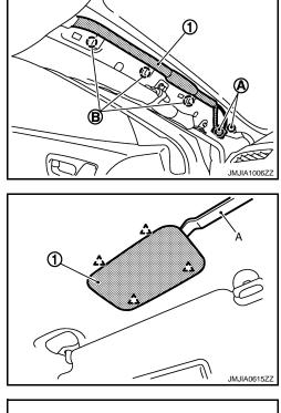
9. Disconnect roof harness connector (A).
