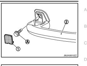
• Remove assist grip (1) with remover tool (A) and then pull back assist grip.
