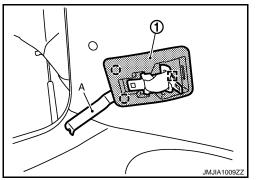
16. Using remover tool, remove headlining hidden clips at the back side of headlining.
