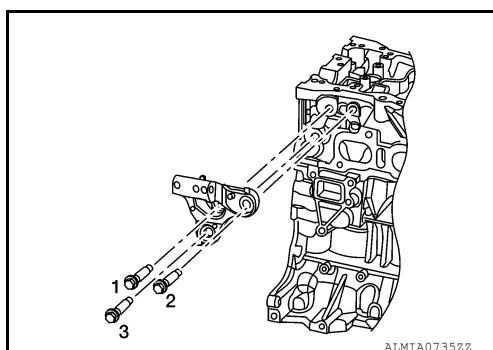
2. Install generator and temporarily tighten bolts in the reverse numerical order as shown.
