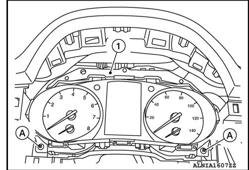
3. Release the clips and remove the combination meter (1) from the instrument panel.
