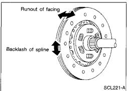
Clutch disc, for backlash of spline and runout of facing Maximum backlash of spline (at outer edge of disc): MODEL 190 0.8 mm (0.031 in) MODEL 215 0.9 mm (0.035 in)
