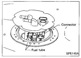
5. Disconnect fuel tube and connector, then remove fuel gauge assembly.
