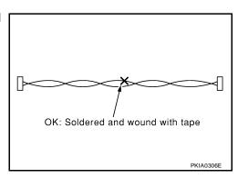
Do not perform bypass wire connections for the repair parts. (The characteristics of twisted line will be lost.)
