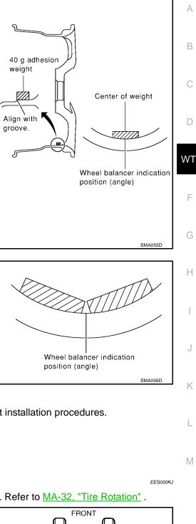
c. If calculated balance weight value exceeds 50 g (1.76 oz.), install two balance weight sheets in line with each other as shown.
