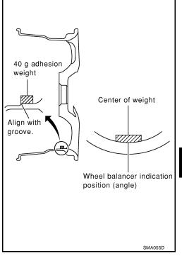
c. If calculated balance weight value exceeds 50 g (1.76 oz.), install two balance weight sheets in line with each other as shown.
