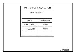
13. WRITE CONFIGURATION results are printed out automatically. Confirm "WRITE CONFIGURATION" is correctly executed by comparing sheet automatically printed out with applicable configuration list shown in step 9.
