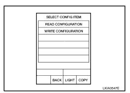
Configuration of current BCM is printed out automatically. A listing of manual setting items and auto setting items will be displayed. Auto setting items are preset and cannot be changed. Manual setting items can be set by using WRITE CONFIGURATION PROCEDURE. Refer to <a href="BCS-16">BCS-16</a>, "WRITE CONFIGURATION PROCEDURE"
