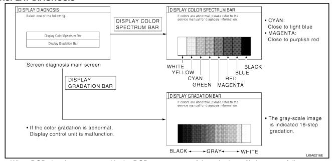
When RGB signal error occurred in the RGB system, tone of the color bar will change as follows.
