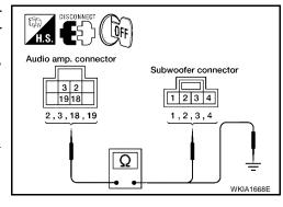
3. Check continuity between BOSE speaker amp. harness connector terminal and ground.
