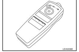
7. Register the IDs in order from FR LH, FR RH, RR RH and RR LH. When ID registration of each wheel has been completed, a buzzer sounds and the warning lamp flashes.
