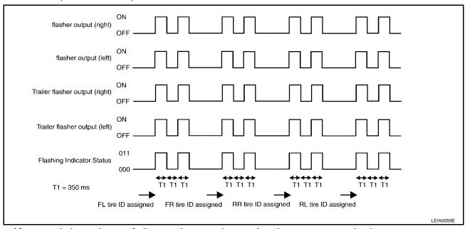
3. After completing wake up of all transmitters, make sure low tire pressure warning lamp goes out.
