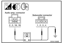
Check continuity between BOSE speaker amp. harness connector terminal and ground.
