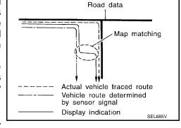
In map-matching, alternative routes to reach the destination will be shown and prioritized, after the road on which the vehicle is currently driven has been judged and the current-location mark has been repositioned.
