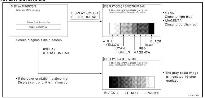
When RGB signal error occurred in the RGB system, tone of the color bar will change as follows.
