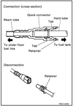
To keep the quick connector clean and to avoid damage and contamination from foreign materials, cover the quick connector with plastic bags or suitable material as shown.
