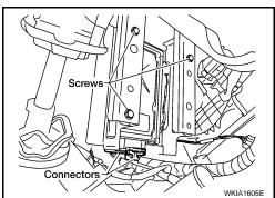
5. Remove the Bose speaker amp.screws (A). then remove the Bose speaker amp. (1).
