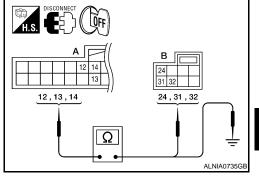
3. Check continuity between Bluetooth control unit connector B142 (A) and ground.
