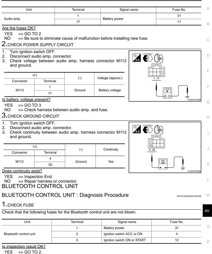
NO >> Be sure to eliminate cause of malfunction before installing new fuse.
