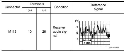
Is the audio signal voltage reading as specified?
