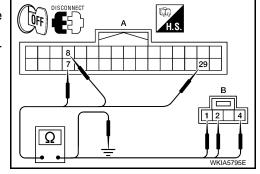
Check continuity between Bluetooth control unit harness connector B142 (A) and ground. 4.
