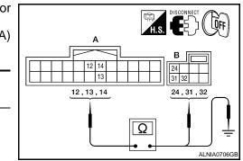
3. Check continuity between AV switch connector M98 (A) and ground.
