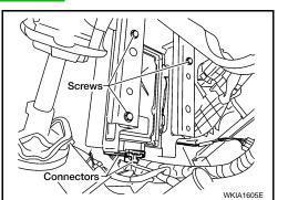
Remove the BOSE speaker amp.screws (A). then remove the 5. BOSE speaker amp. (1).
