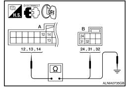
3. Check continuity between Bluetooth control unit connector B142 (A) and ground.
