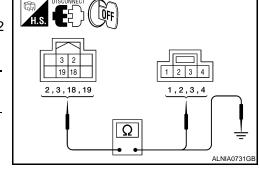
3. Check continuity between audio amp. harness connector M112 (A) and ground.
