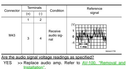
NO >> Replace audio unit. Refer to <u>AV-92. "Removal and</u> <u>Installation"</u>.
