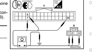
4. Check continuity between Bluetooth control unit harness connector B142 (A) and ground.
