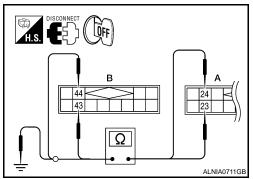
4. Check continuity between satellite radio tuner (factory installed) connector M41 (A) and ground.
