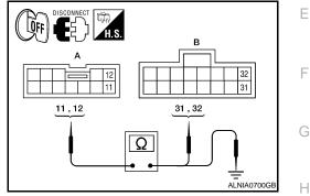
4. Check continuity between video monitor harness connector R202 (A) and ground.
