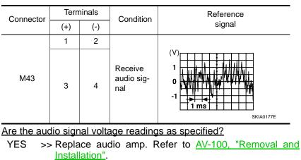
NO >> Replace audio unit. Refer to <u>AV-92, "Removal and</u> <u>Installation"</u>.
