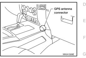
5. Remove the GPS antenna.
