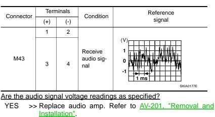
NO >> Replace audio unit. Refer to <u>AV-189</u>, "<u>Removal and</u> <u>Installation</u>".
