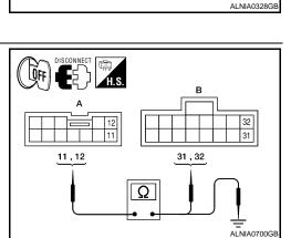
4. Check continuity between video monitor harness connector R202 (A) and ground.
