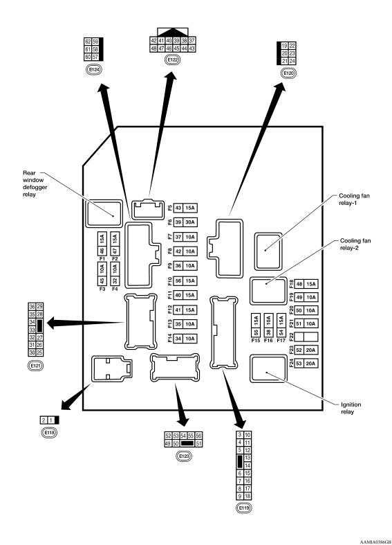
Numbers preceded by an "F" represent the fuse numbers imprinted on the IPDM E/R. The other numbers represent the fuse numbers as they appear in the wiring diagrams.
