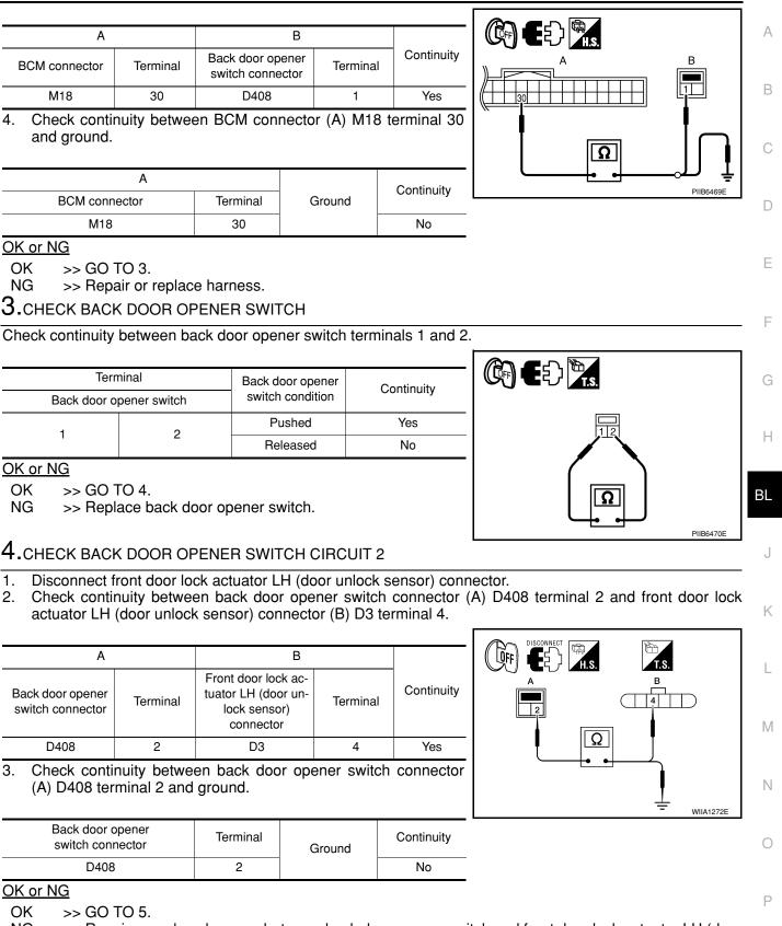
NG >> Repair or replace harness between back door opener switch and front door lock actuator LH (door unlock sensor).
