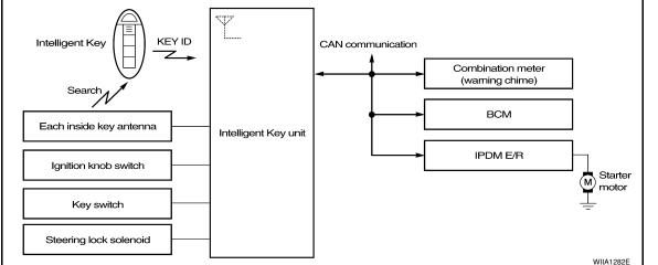
When ignition knob switch is ON (press ignition switch), Intelligent Key unit searches Intelligent Key in the vehicle using inside key antenna.
