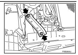
Tie a cord to all radiator core upper supports of the radiator and condenser.
