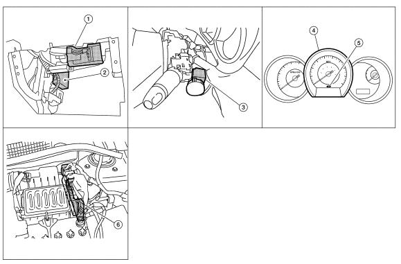
1. BCM M18, M19, M20 (view with glove box removed)
