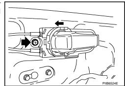
7. Disengage the handle from the door panel, and remove the inside handle.
