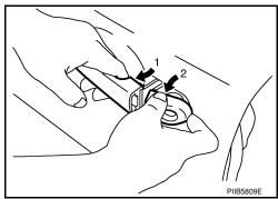
7. Pull outside door handle forward (1), and slide it toward the rear of the vehicle to remove (2).
