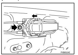
Disconnect the inside handle and lock knob cables from the 4. inside handle. **CAUTION:**
