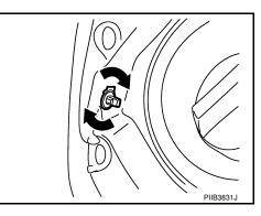
5. Remove fuel filler lid opener cable clip from the vehicle.
