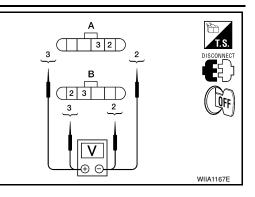
Check voltage between rear door lock actuator connector LH (A) D205 or rear door lock actuator connector RH (B) D305 terminals 2 and 3.
