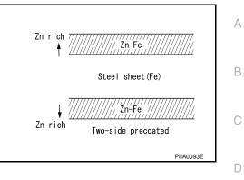
Nissan Genuine Service Parts are fabricated from galvannealed steel. Therefore, it is recommended that GENUINE NISSAN PARTS or equivalent be used for panel replacement to maintain the anti-corrosive performance built into the vehicle at the factory.
