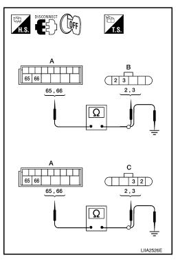
4. Check continuity between BCM connector (A) M20 terminals 65, 66 and body ground.
