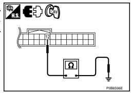
Key Switch (Intelligent Key Unit Input) Check
