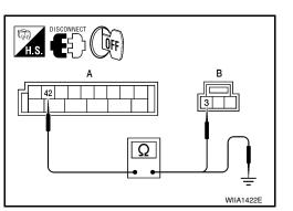
3. Check continuity between BCM harness connector M19 (A) terminal 42 and ground.
