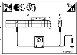
3. Check continuity between Intelligent Key unit connector and ground.
