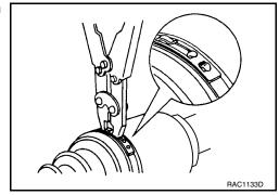
10. Install new small boot band securely using Tool.
