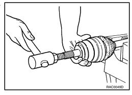
Insert the balance of new grease (Genuine NISSAN Grease or equivalent) listed below into housing from large end of boot.
