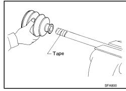
3. Align matching mark on spider assembly with matching mark on shaft and install spider assembly with chamfer facing shaft.
