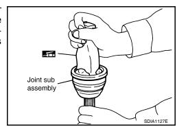
2. Cover serrated part of shaft with tape. Install new boot band and new boot to shaft.
