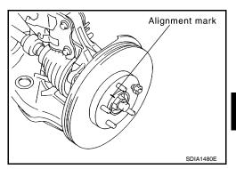
Remove wheel sensor from steering knuckle. Refer to BRC-32. **CAUTION:**
