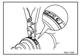
Secure boot band so that dimension (M) meets specification as shown.
