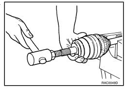
Insert the balance of new grease (Genuine NISSAN Grease or equivalent) listed below into housing from large end of boot.
