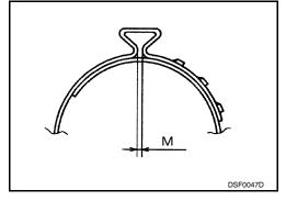
11. Rotate the slide joint and confirm that the boot position is correct. If boot position is not correct, remove the boot bands, reposition the boot and install new boot bands.
