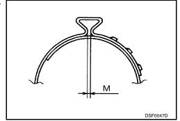
9. Rotate the joint sub assembly and confirm that the boot position is correct. If boot position is not correct, remove the boot bands, reposition the boot and install new boot bands.
