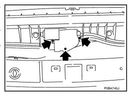
6. Remove the side and front sunroof unit assembly nuts.
