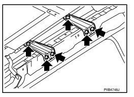
7. Connect the sunroof motor assembly connector and install the screws.
