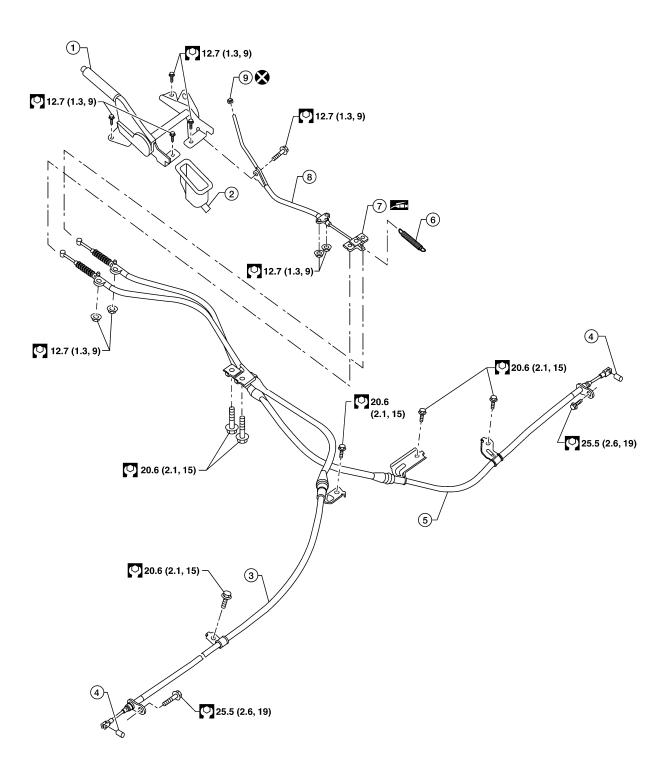
WFIA0406E Control lever assembly 2. Front cable grommet 3. Left rear cable 1. 4. Pin 5. Right rear cable 6. Return spring 8. 7. Equalizer Front cable 9. Adjusting nut
